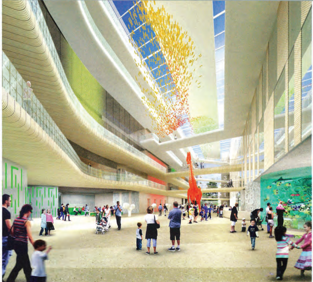
Figure 3. Oriented north and flooded with daylight, the wayfinding main street has a thermal labyrinth and natural ventilation.
